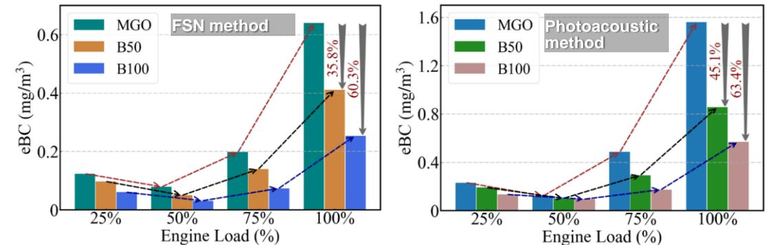
Source: IMO PPR 10/Inf.4, January 30, 2023, Black carbon emission measurement results of a marine low speed diesel engine using biofuel.
